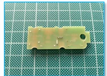
Next fit the switch. It does not matter which way up, but it must be fitted close to the PCB and will sit in the little cut-out. It will be easier if you tin the three switch pins before soldering to the PCB.
