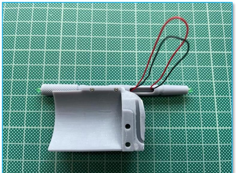
After soldering, slide up the heat shrink tubing over the connections and shrink with hair dryer or heat gun.
