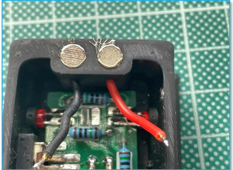
Next you need to solder the wires to the PCB pads. Ensure the correct polarity. You may find that tweezers help hold the wires for soldering. It is also advisable to tin the pads before trying to attach the wires.
